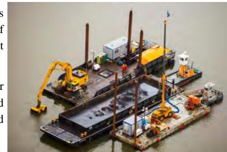
Instrumented Fixed Arm Excavator Dredge
