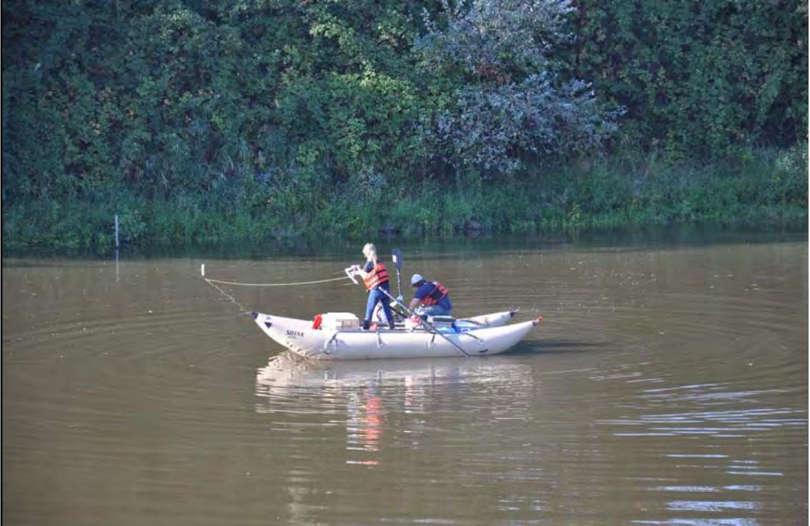
Employees of Apex Companies, LLC and Texas Tech University deploy passive sediment porewater sampling equipment in the Lower Columbia Slough (Portland, Oregon). The sampling was performed in preparation for sediment remediation as a baseline for evaluation of activated carbon amendment performance.
