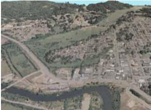
Highest hit and bare earth lidar images can be rendered in 3-D to help land use planners and others visualize topography with much greater detail than ever before. Image of Coquille, Oregon."
