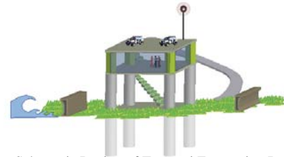
Schematic Design of Tsunami Evacuation Building (TEB)
